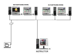
The simulation models are developed on the state-of-the-art "ProSimulator" dynamic simulator. ProSimulator is an integrated dynamic simulation environment consists of Instructor station s/w, real-time database, operator station emulation s/w, interface s/w to DCS and dynamic simulation development package.
