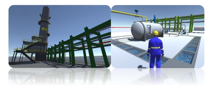
The package consists of 3D simulation models for various units and plants. Each model simulates respective units and the field operations with its local control panel, associated filed instrumentation and safety systems. The Instructor can invoke malfunctions, disturbances and instrument failures and evaluate the trainee performance.
